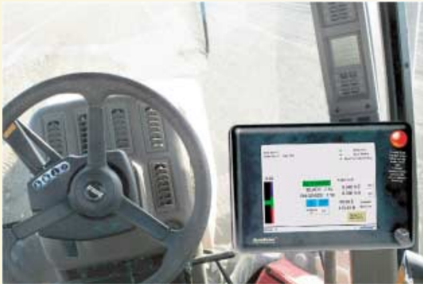
The AutoLevel system is controlled by a touch screen mounted in the tractor cab.
