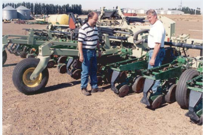
Watts Brothers 100 Circles Farm managers Blake Hatch (L) and Todd Clark with the business end of the Orthman 12-row planter used with AutoFarm's AutoSteering system to plant corn. (photo taken 9102)
